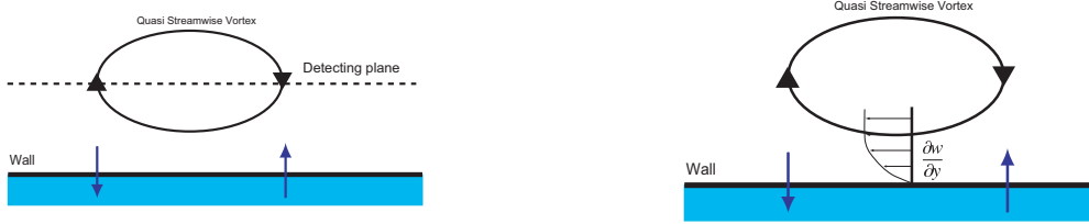
Figure 3.12: Schematics of control schemes: left, v -control (Choi et al., 1994); right, suboptimal control (Lee et al., 1998).
