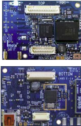
Figure 1: Intel's Imote2. Top view (top) and bottom view (bottom) [5].
